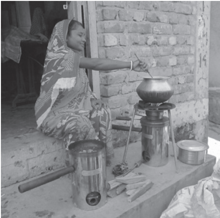
A micro-gasifier stove in West Bengal, India, to cook food and create charcoal.
